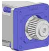
6. Center the adapter onto the motor flange and screw up.
