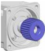
3. Push the gear wheel on until it touches the spacer washer on the drive pin.
