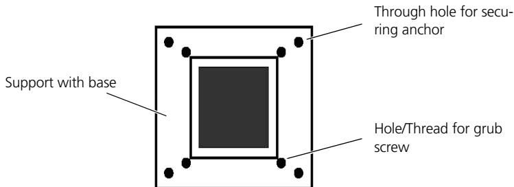
Unevenness of the Type 1 (Clamp element Type FVV) foot construction can be levelled out using the grub screws Protective shims placed under the feet prevent the ends of the grub screws digging into the base. The adjusting shims allow full surface support of the foot clamping piece on uneven bases.
