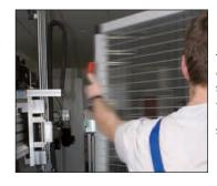
The locking system is activated when the machine is at a standstill, preventing the Z axis from lowering vertically. It is now safe to enter the safety zone.
